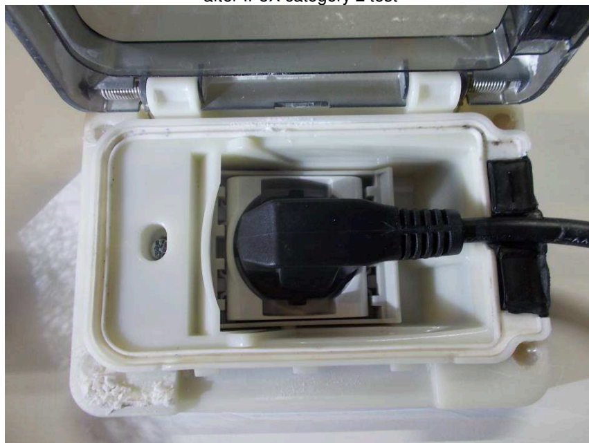
Naked eye visual internal inspection on built in mounting box after IP5X category 2 test
