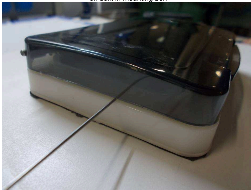
IP 5X category 2 test (wire test) on built in mounting box
