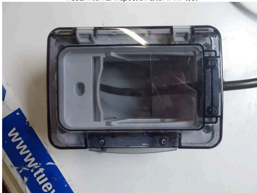
Visual internal inspection after IPX7 test
