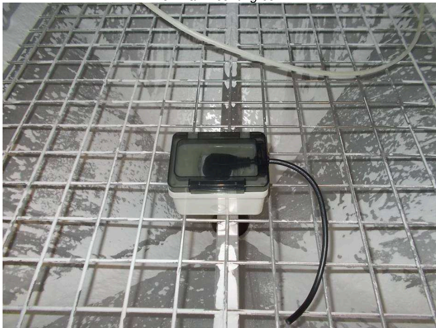
IP 5X category 2 test on wall mounting box
