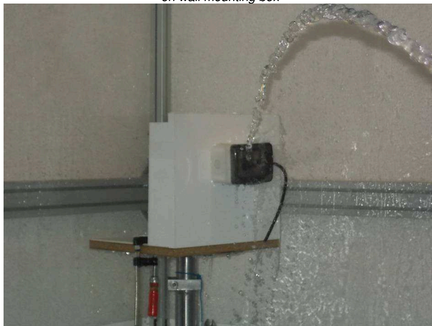
Naked eye visual internal inspection after IPX5 test on wall mounting box
