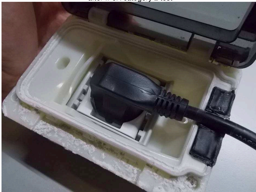
Naked eye visual internal inspection on wall mounting box after IP5X category 2 test
