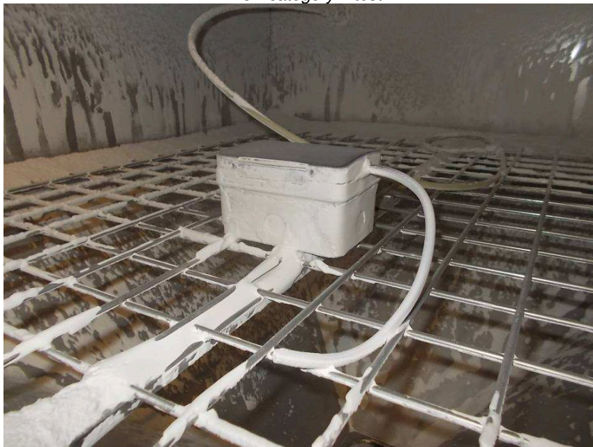
Naked eye visual internal inspection on wall mounting box after IP5X category 2 test
