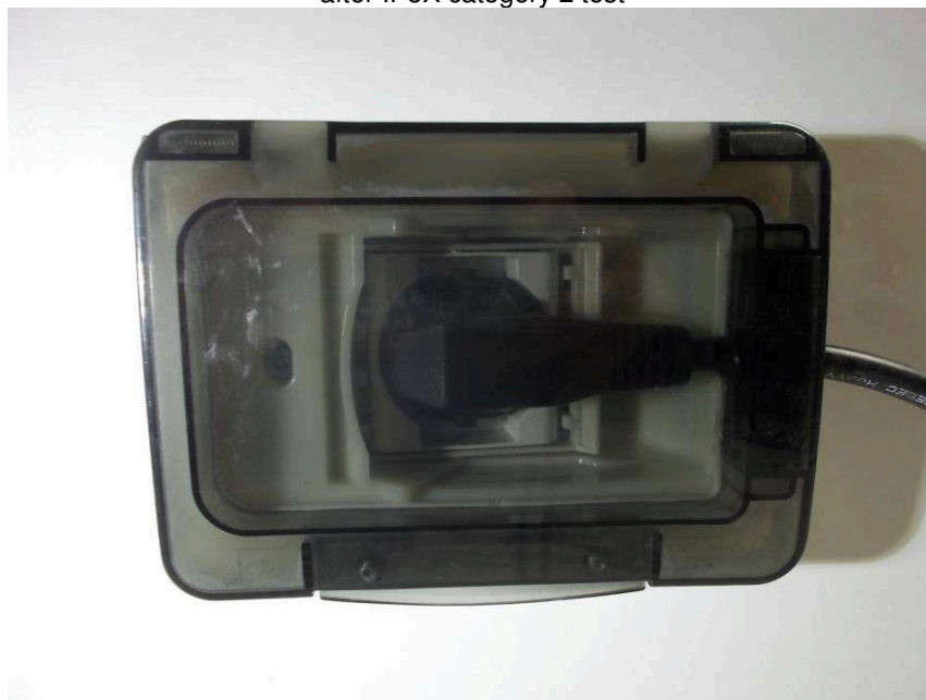
Naked eye visual internal inspection on built in mounting box after IP5X category 2 test
