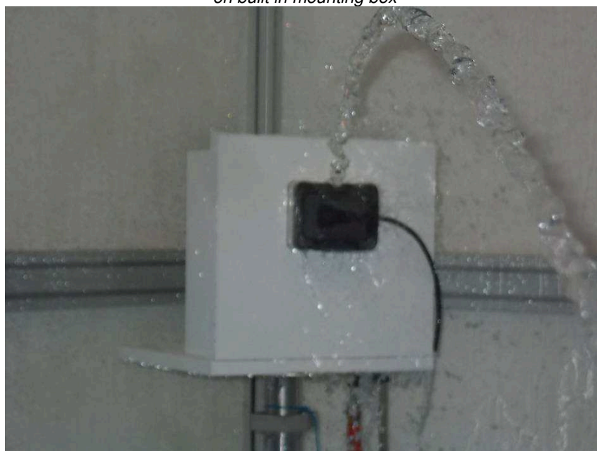
IP X5 test on built in mounting box
