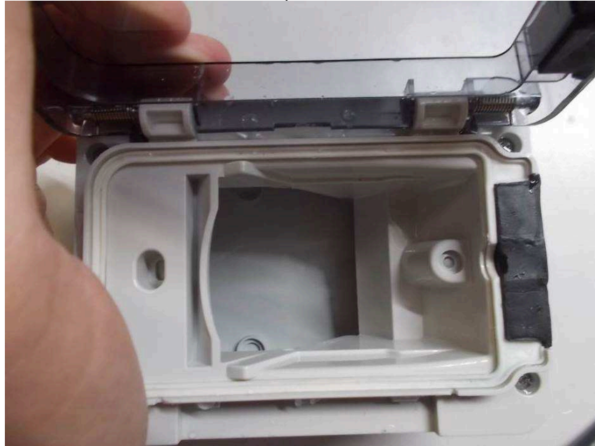
Visual internal inspection after IPX7 test
