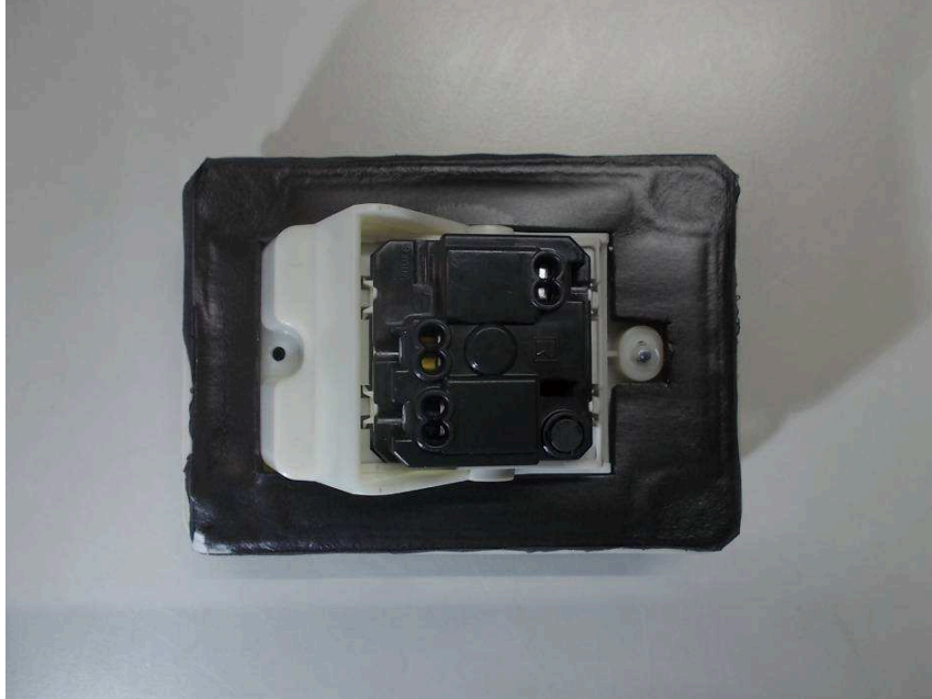
Naked eye visual internal inspection after IPX5 test on built in mounting box
