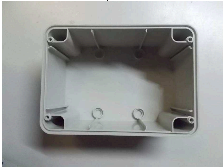
Visual internal inspection after IPX7 test
