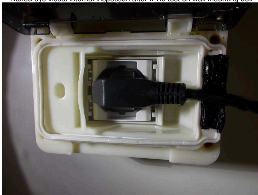
Naked eye visual internal inspection after IPX5 test on wall mounting box
