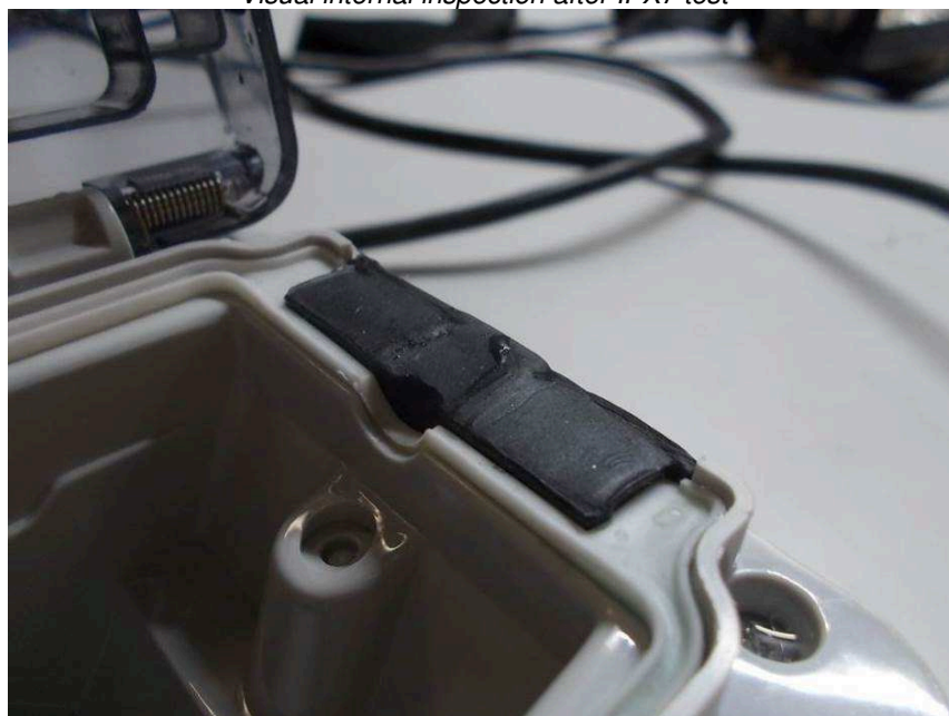
Visual internal inspection after IPX7 test
