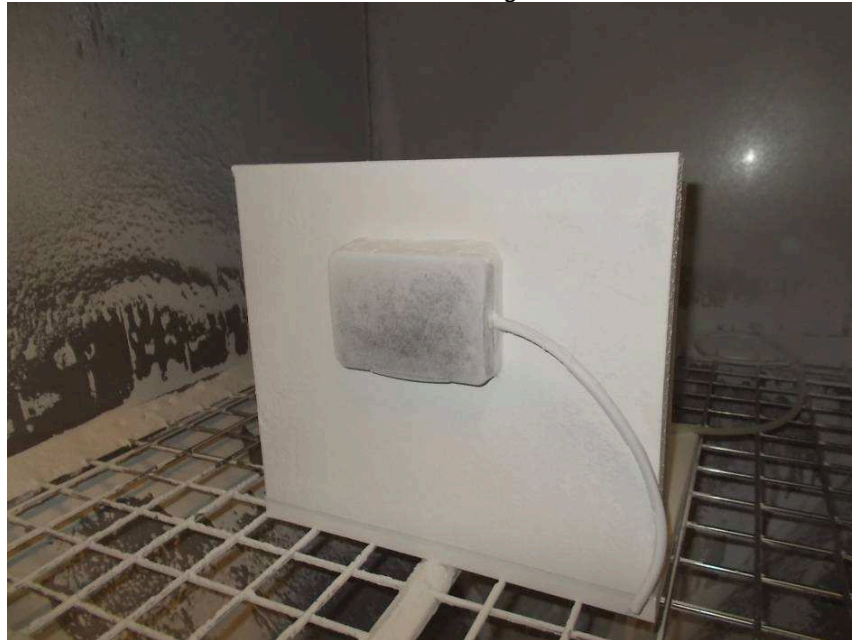
IP 5X category 2 test on built in mounting box
