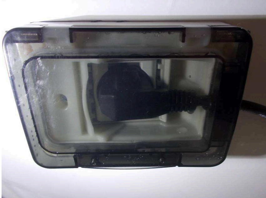
Naked eye visual internal inspection after IPX5 test on built in mounting box (water drop detail)
