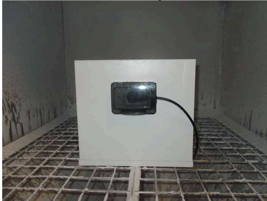
IP 5X category 2 test on built in mounting box
