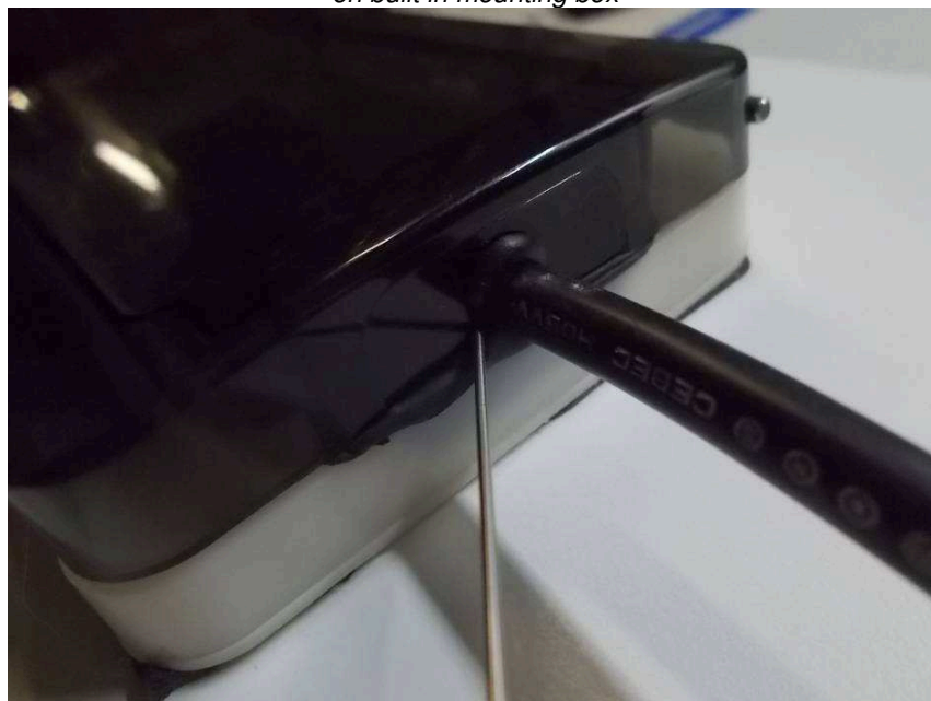
IP 5X category 2 test (wire test) on built in mounting box
