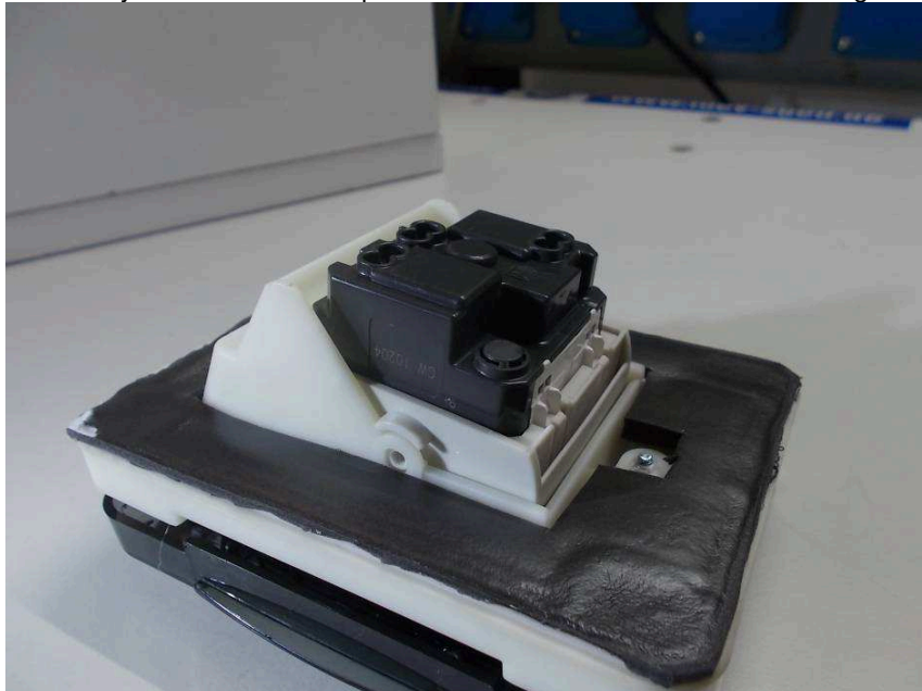
Naked eye visual internal inspection after IPX5 test on built in mounting box
